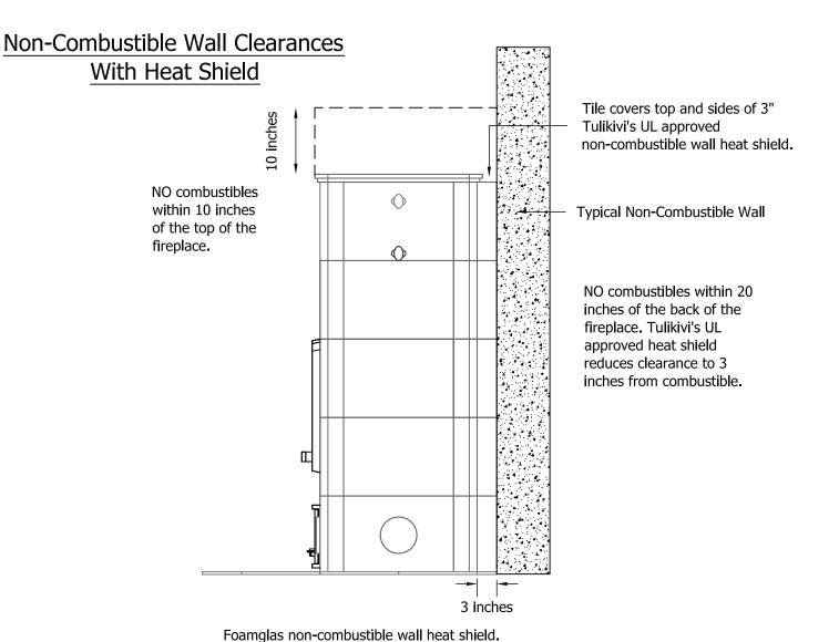
If a foamglas heat shield is not present between the fireplace and the non-combustible wall you must maintain 14" from sides and 20" from the back of the fireplace to combustibles.
