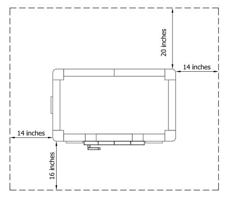
NO combustibles within 20 inches of the back of the fireplace. Tulikivi's UL approved heat shield reduces clearance to 3 inches from combustible.
